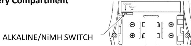
2. Install the AA batteries. Be sure to observe proper polarity (+/-). Damage due to improper installation may void the warranty on the product. The “Power On” LED on top of the unit will flash when the batteries are getting low; you may continue to use until the unit quits operating, then replace or recharge the batteries (FIG A)
